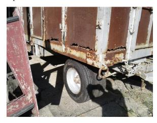
Once we can get it wire brushed down and primed, we can start working on putting the wings back on the wagon. Our good friend, Dominic Yodice explained that the wings were made out of 1" steel angle iron with a <sup>3</sup>/<sub>4</sub>" piece of plywood inside. This gave a very small lip which was just enough to keep a band member's chair from going over the edge.
